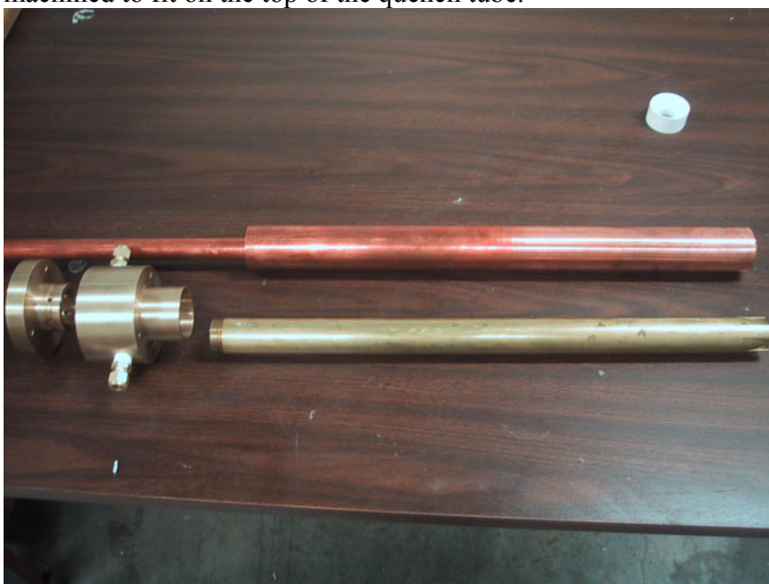
Figure 4: Disassembled quench tube
