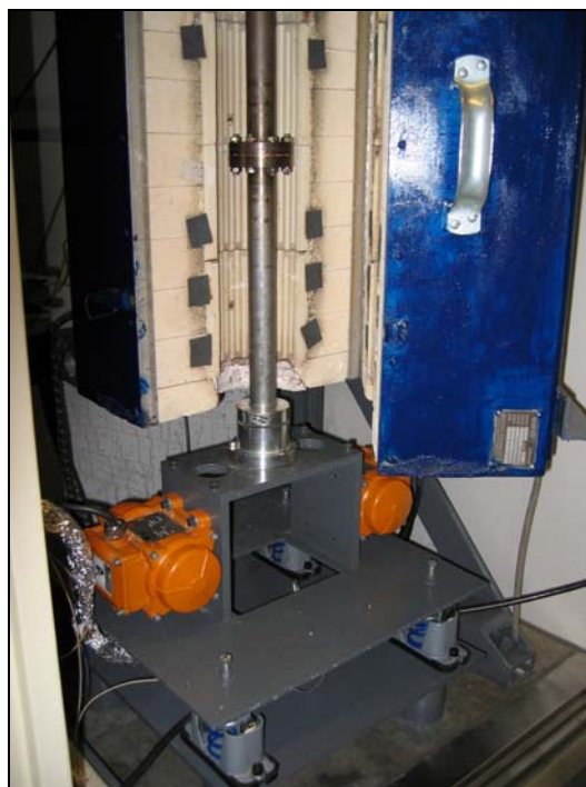
Fig. 1. (a) Schematic of fluidization apparatus: 1) Fluidization column, 2) vibro-motors, 3) spring supports, 4) pressure transducers, 5) sintered-metal filter. (b) System detail.
