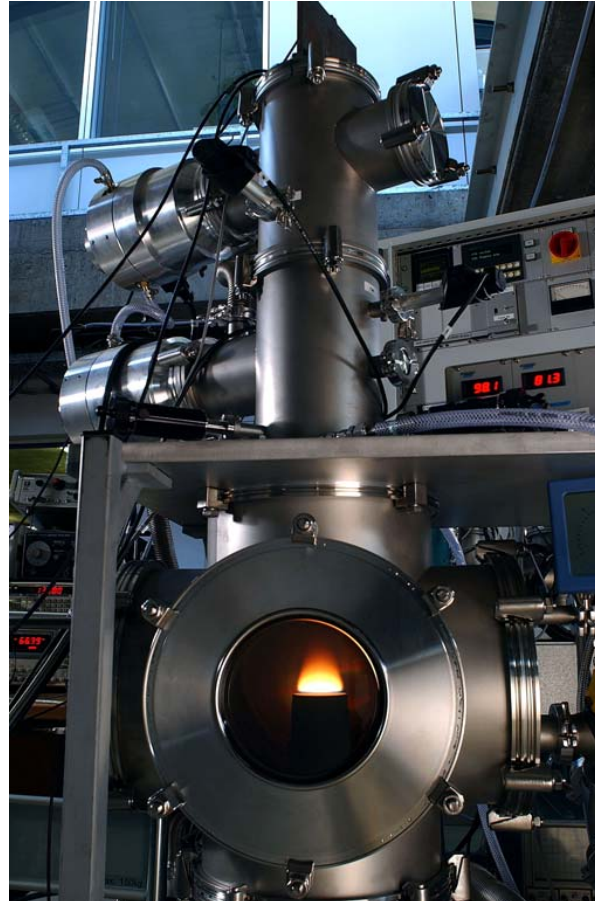
Fig. 1: Particle Mass Spectrometer attached on top of low pressure burner chamber.
