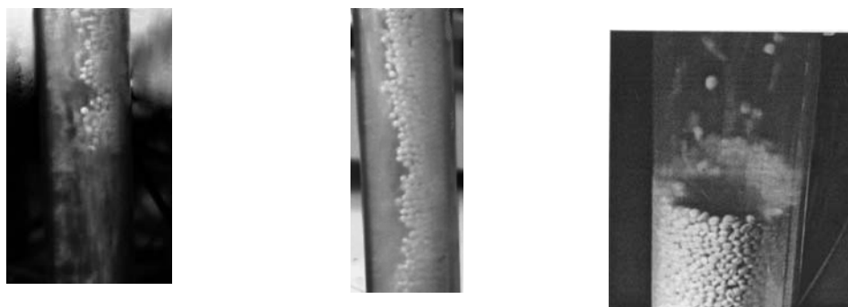
Figure 2. Three typical granular flow patterns at vertical pipe with air flow rate (a) > 1200 liters/min; (b) 900\sim 1150 liters/min; (c) < 860 liters/min.
