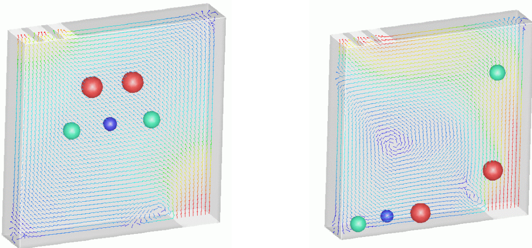
Figure 4. Particle motion in a box. Airflow is from bottom right to top left.
