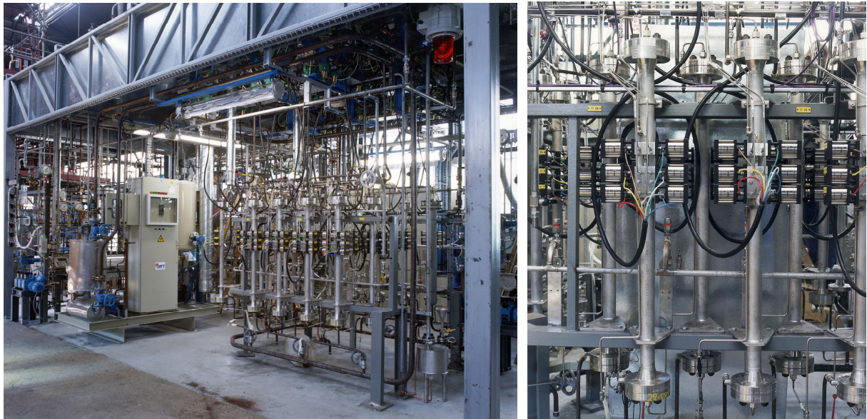
Figure 4 : general view of the pilot plant and a detailed view of the on / off valves system.
