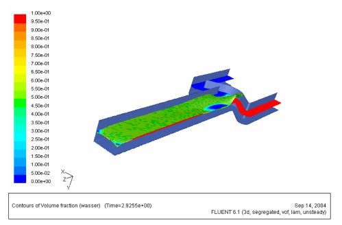
*Figure 9:* Calculated unsteady state interface for700 x 700 µm cross section of the micro channel
