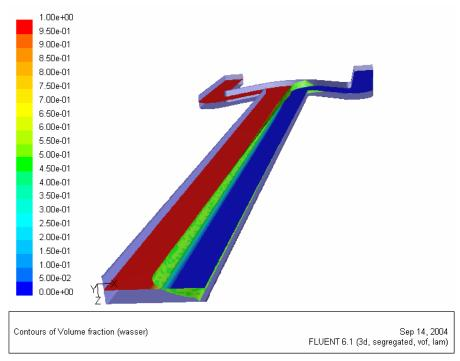
Figure 8: Calculated steady state interface for 700 x 200 µm channel width
