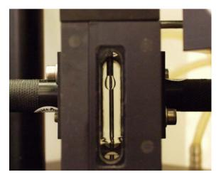
Figure 5: Interfacial tension measurement system (growing water droplet)
