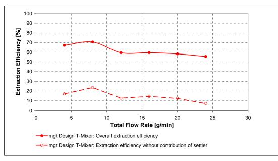
*Figure 3:* Total flow rate dependence of the overall extraction efficiency and the extraction efficiency without contribution of the settler (broken lines) respectively at constant phase ratio of feed and solvent of 1 for the *mgt Design T-Mixer* microreactor; T=293 K
