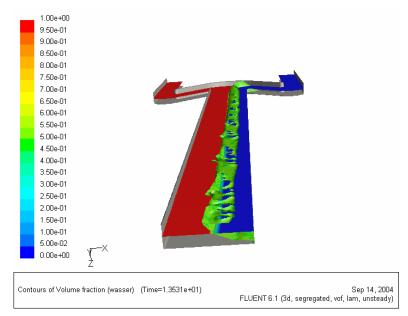
Figure 7: Calculated interface after 13.51 sec (700 x 200 µm)
