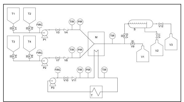
Figure 2: Experimental setup of the microplant: (T1) Feed storage tank, (T3) Solvent storage tank, (T3, T4) Purge tanks, (P1) Feed pump, (P2) Solvent pump, (P3) Pump for heat transfer medium, (T) Cryostat, (M) Microreactor, (S) Settler, (V1) Waste vessel, (V2) Raffinate vessel, (V3) Extract vessel, (V1, V2, V5, V6, V9, V10) Solenoid valves, (V3, V7, V10) Pressure control valves, (V4, V8, V11) Check valves, (V11, V12) Valves
