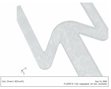
Figure 6: Grid construction of the microchannel with feed channels (700x200µm)
