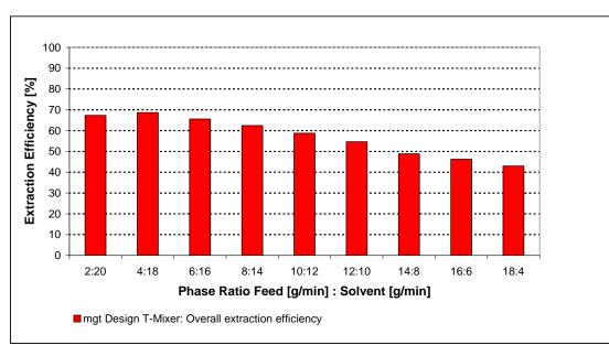
*Figure 4:* Dependence of varying phase ratio of feed and solvent on the overall extraction efficiency at constant total flow rate of 22 g/min for the *mgt Design T.Mixer* microreactor; T=293 K
