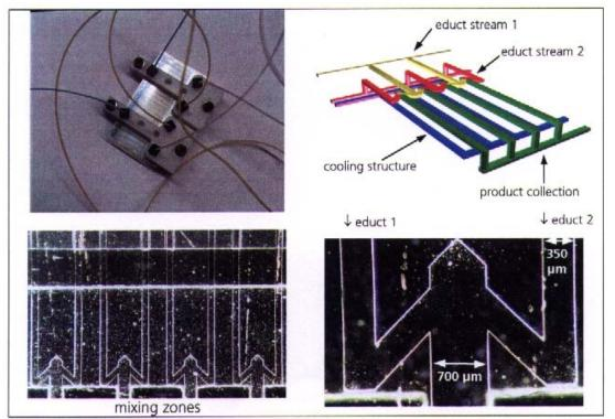
*Figure 1:* Construction principle of the investigated micromixer with schematic flow and microscopic image of the inlet microchannels
