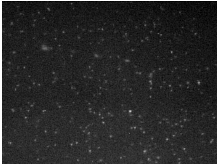
Figure 9, Primary Nucleation seen by Crystal Microscope Process Camera
