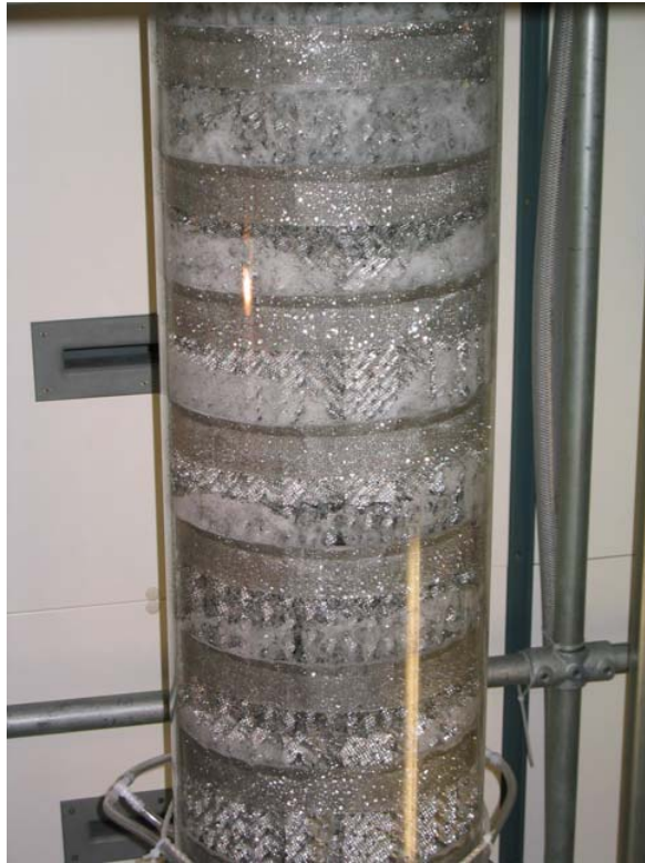
Figure 5. Flooded SULZER Mellapak 305.Y, B = 15 \text{ m}^3/\text{m}^2\text{h} , F = 1,9 \text{ Pa}^{1/2}
