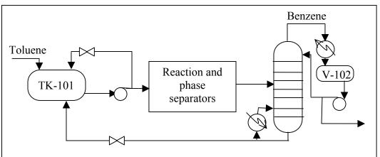
Figure 5: Diagram of the hydrodealkylation unit
