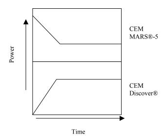
**Figure 2.** Schematic of the power versus time plot observed for MARS®-5 multi-node microwave oven and Discover® single-node microwave oven
