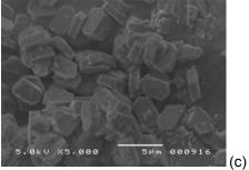
**Figure 1.** Scanning electron micrographs of silicalite from microwave synthesis with (a) 2 min ramp, 10 hold at 175°C, (b) 120 min ramp, 10 hold at 175°C and (c). 2 min ramp, 128 hold at 175°C
