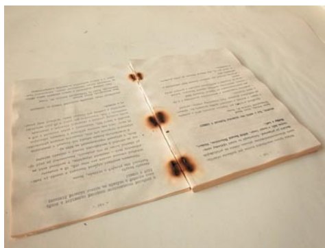
Figure 4. Example of document damage by red-heating of metal staples in a batch dryer
