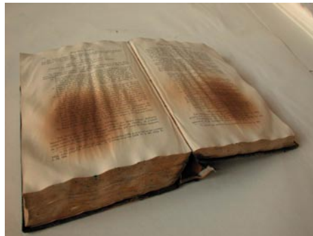
Figure 3. Example of document damage by overheating and hot-spots in a batch dryer
