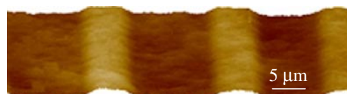
Figure 7 AFM image of copper film electroplated on patterned silicon wafer.
