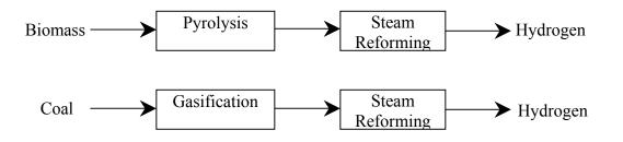
Figure 1 Conversion Process from Biomass and Coal to Hydrogen
