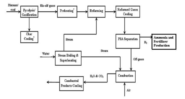
Figure 3 Whole Conversion Process from Biomass and Coal to Hydrogen and Fertilizer
