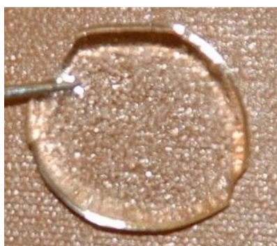
Fig. 1. Digital image of a membrane prepared using Brij 22 and \text{CF}_3\text{SO}_3\text{H} .
