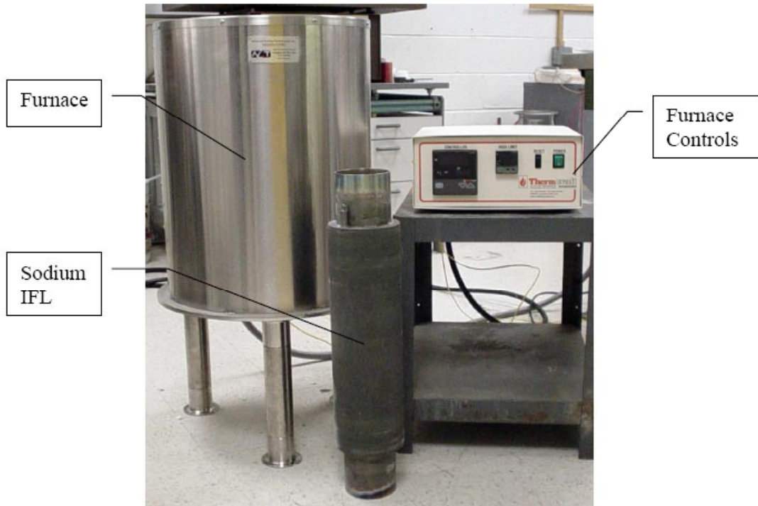
Figure 2: The Sodium Isothermal Furnace Liner being displayed outside the Furnace
