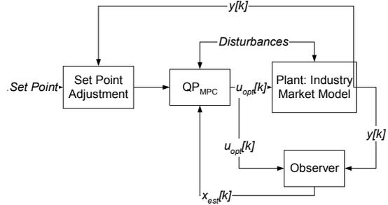
Fig. 3. The Implemented MPC Controller (Morari et al., 1998)
