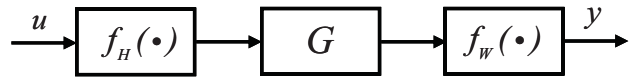
Figure 6. General Hammerstein-Wiener model structure; f_H is the Hammerstein static nonlinear transformation, f_w is the Wiener static nonlinear transformation.
