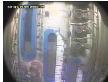
Fig. 2. Separation cell with three side view glasses
