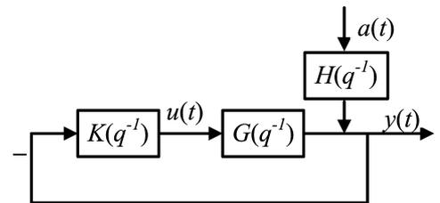
Fig. 2. Block diagram of closed-loop system
