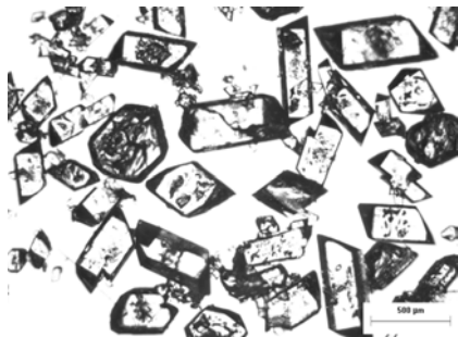
Fig. 11. Microscopy image of paracetamol product crystals for the unseeded system using C-control.
