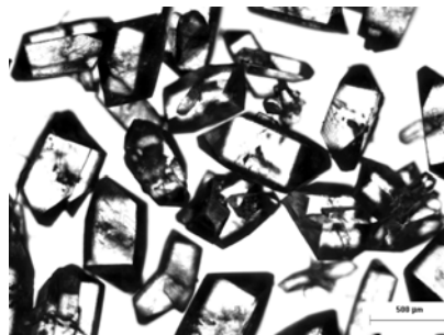
Fig. 13. Microscopy image of paracetamol product crystals for the seeded system using C-control.
