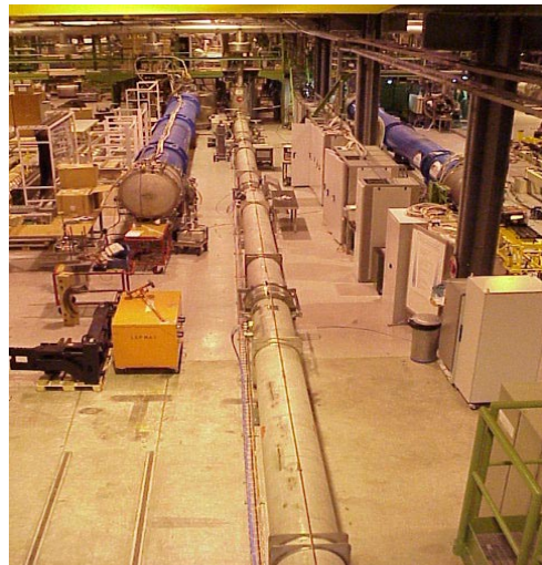
Fig. 1 Inner Triplet Prototype (length: 30 meters)
