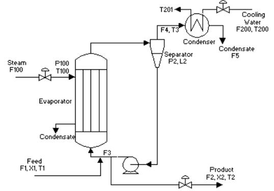
Fig. 1. Evaporator System
