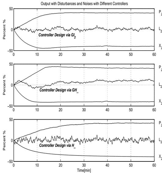
Fig. 3. Response to Step Changes in Setpoints
