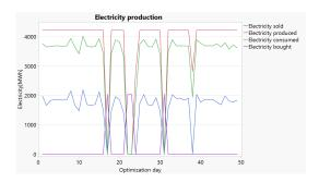
Fig. 5. Electricity produced and sold in Period 1. The red line represents the total amount of energy produced from the CCGT, the green one the part not transformed into steam. Blue and violet line are, respectively, the electricity sold and bought on the market
