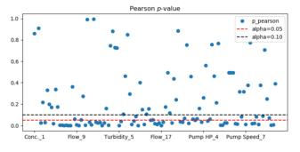
Figure 7 – P-values of the Pearson's correlation of process data from the flotation unit and the toxin level.
