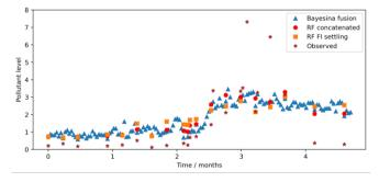
Figure 10 - Time series plot of observed and predicted toxin levels for various methods using fluid image data from settling unit (RF FI settling), concatenated RF, and Bayesian fusion.
