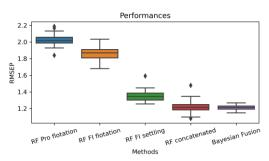
Figure 9 - Test results for the single-source (RF Pro Flotation - RF using the Process data from Flotation unit; RF FI flotation - RF derived from imaging data from the Flotation unit; RF FI settling – RF using data from settling unit) and multi-source (RF Concatenated and Bayesian Fusion).
