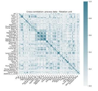
Figure 6 - Heatmap of absolute value of Pearson's correlation coefficient between predictors, process data from flotation unit.
