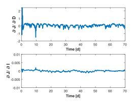
Fig. 10. ML-ES application with noise corrupting the input/output signals: evolution of the gradient components.
