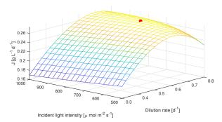
Fig. 3. Steady-state map showing the biomass productivity J as a function the inputs D and I. The red star indicates the optimum.
