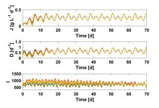
Fig. 6. RLS-ESC application: evolutions of the inputs and output. Optimal values are shown by the dashed lines.
