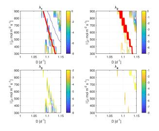
Fig. 4. Contours of the evolution of the eigenvalues of the Jacobian of f(x):  $\lambda_1$  to  $\lambda_4$  are respectively related to X, S, Q and  $I^*$ . The red zones represent the positive contours (unstable regions), separating the  $\lambda_1$  and  $\lambda_2$  diagrams in two stable regions.
