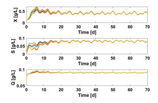
Fig. 7. RLS-ESC application: evolutions of the biomass, substrate and internal quota concentrations.
