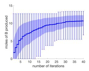
Fig. 2. The maximum performance (moles of B) versus number of BO iterations for 100 replicate runs. The dark blue line represents the mean value, the shaded region is +/- one standard deviation, and the error bars show the minimum and maximum values.
