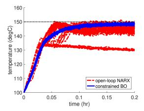
Fig. 4. Closed-loop temperature profile obtained using the proposed constrained BO method compared to an open-loop identified NARX model in the presence of measurement noise for 100 Monte Carlo realizations.
