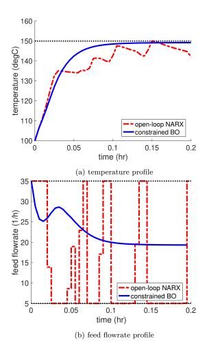
Fig. 3. Closed-loop (a) output and (b) input profiles for best solution obtained with BO compared to an openloop identified NARX model for the noise-free case.
