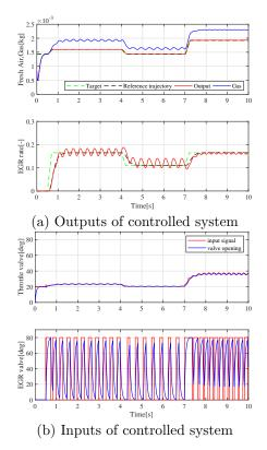
Fig. 3. Simulation results of the method without antiwindup compensation
