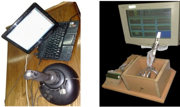
Fig. 4. Master and Slave sides used in practical experiment, the left picture shows the master side and the right picture shows the slave.
