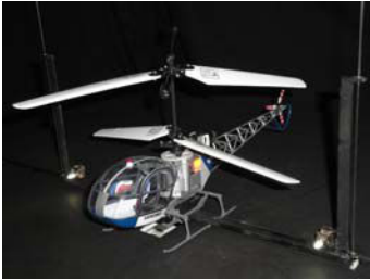
Fig. 3. Photograph of XRB SR lama with two LEDs constrained by two vertically directed parallel wires
