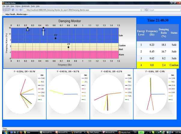
Fig.8 Snapshot Example of a Damping Monitor Webpage
