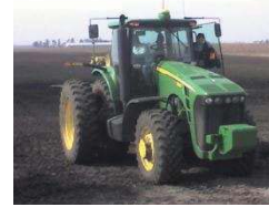
Fig. 6. Experiments are conducted on a John Deere tractor with integrated AutoTrac™ (model 8330, Deere and Co.).
