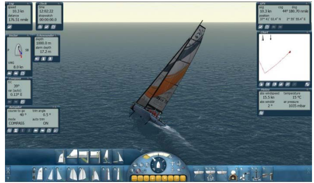
Fig. 6. Picture of the simulation environment that highlight the command line (on the bottom) and analog and digital indicator on the right and left hand.
