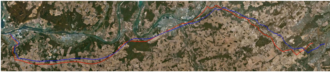
Fig. 6. Comparison of estimated trajectory (blue) with GPS (red). The approximate path length is 80 km. obtained during a 80 min. trip.
