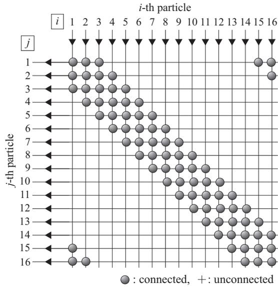
Fig. 1. Information flow in cyclic-network topology for the case of  $n_p = 16$  and  $n_s = 4$
