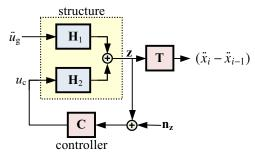
Fig. 3. Control system with state feedback measurement noise.
