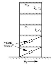
Fig. 1. A shear structure with a VSDD brace control system.
