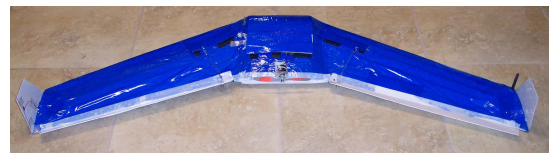
Fig. 5. The MAV flown in flight tests is shown. The wing span is 48 inches with elevons for control surfaces.
