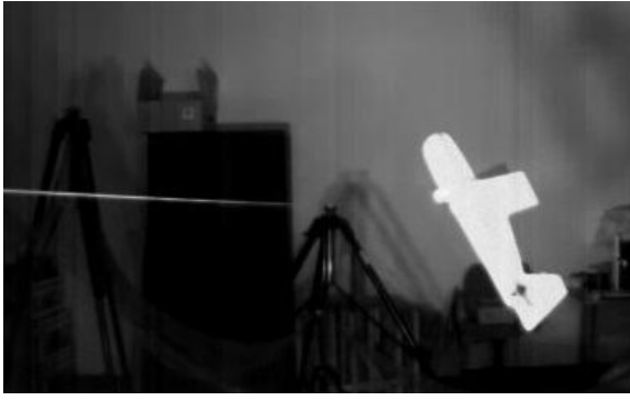
Fig. 2. A image taken with a high-speed camera from one of the perching trajectories used to obtain data on lift and drag coefficients. The target perch can be seen in the left of the image.
