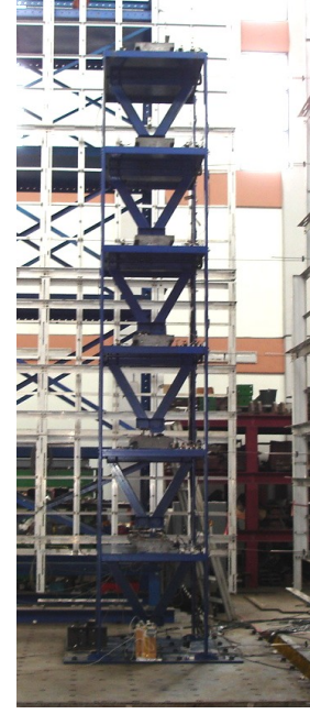
Fig. 1. Six-story test structure.
