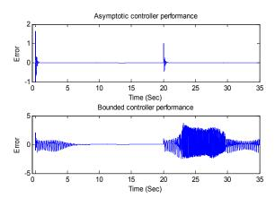
**Figure 2:** Tracking error for the reference trajectory 2 by the asymptotic and the bounded NN controllers.
