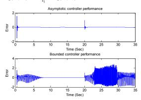
**Figure 1:** Tracking error for the reference trajectory 1 by the asymptotic and the bounded NN controllers.
