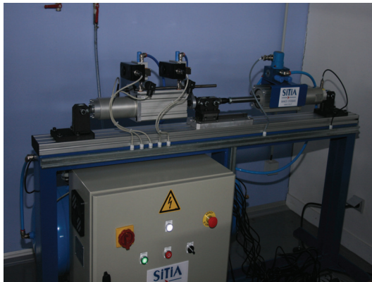
Fig. 1. Photo of the electropneumatic system - On the left hand side is the “main” actuator whose its position is controlled. On the right hand side is the “perturbation” actuator whose the load force is controlled.
