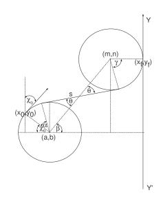
Fig. 2. Dubins' RSL path for initial orientation  $(\chi_0) < \pi/2$  and final orientation  $(\chi_f) = 0$ .
