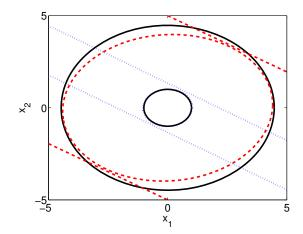
Fig. 1. Reachable sets and input constraints: The inner and outer solid ellipsoids represent  $x^T \Gamma x \leq \delta_x$  and  $x^T \Gamma x < \varepsilon$ , respectively. The dotted ellipsoid and lines represent a reachable set  $\mathcal{E}_0$  from (25) and an input constraint  $|Fx| \leq 2.0$  by Corollary 3.1 at  $\mathcal{N} = 0$ . The dashed ellipsoid and lines represent  $\mathcal{E}_5$  and  $|Fx| \leq 7.0$  by Corollary 3.1 at  $\mathcal{N} = 5$ .
