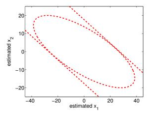
Fig. 2. Reachable sets of the estimated state and input constraints: The dashed ellipsoid and lines represent a reachable set  $\mathcal{E}_2$  from (32) and an input constraint  $|Fx| \leq 27.0$  by Corollary 4.2 at  $\mathcal{N} = 2$ .
