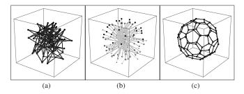
Fig. 2. Execution of the coordination algorithm (8) with h = .25 over a relative sensing network in  $\mathbb{R}^3$  composed of 60 agents. (a) shows the initial configuration, (b) shows the evolution, and (c) shows the final formation.
