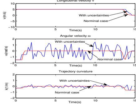
Fig. 5. Control variables and trajectory curvature
