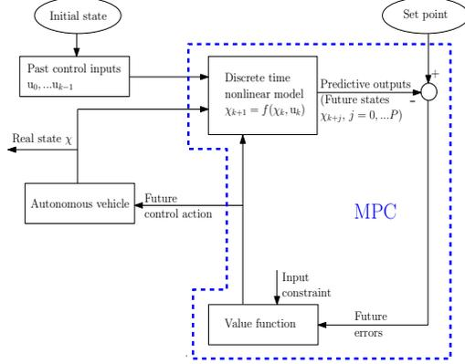
Fig. 3. Control architecture
