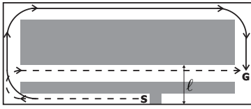
Fig. 1. Counterexample for path planning without kinematic constraint.
