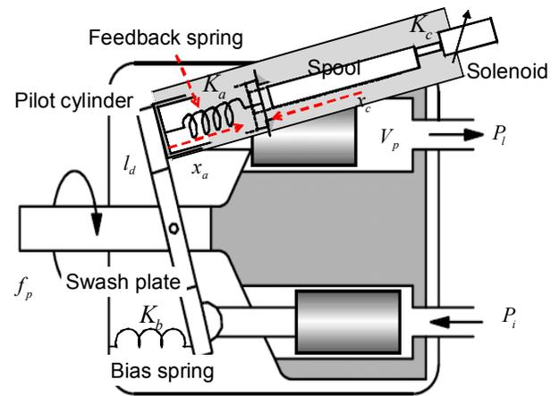
Fig. 2. Basic axial pump diagram.
