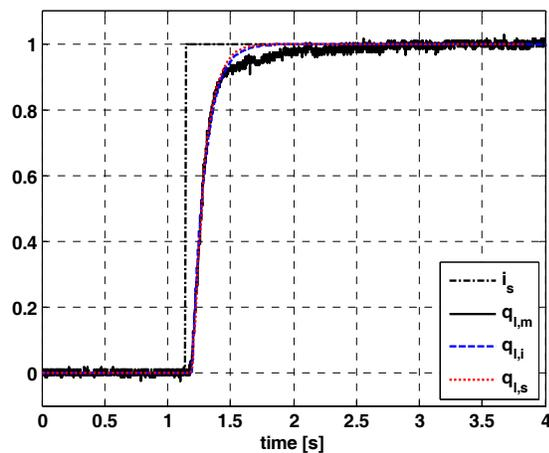
Fig. 5. Pump responses, measured and identified.
