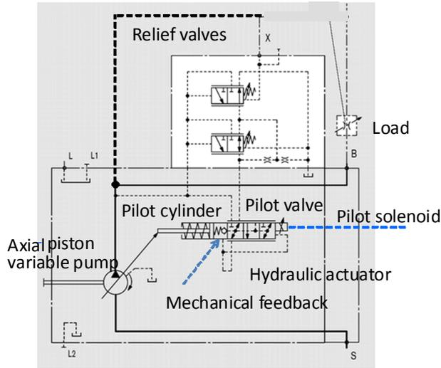
Fig. 1. Essential hydraulic circuit.
