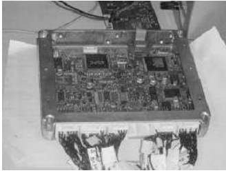
Fig. 2. Engine Control Unit with the embedded controller software.
