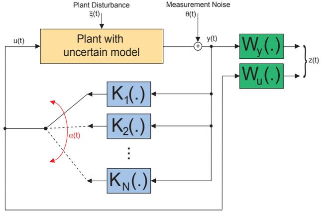
Fig. 1. Feedback interconnection between the plant (1) and the controllers  $K_i$ , selected through signal  $\alpha(t)$ .
