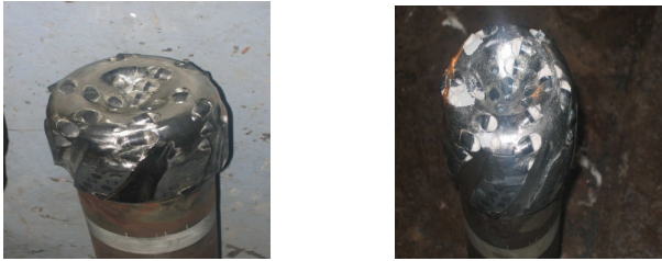
Fig. 2. Drill bit – on the left without balling – on the right with balling
