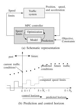
Fig. 2. Conceptual representation of model predictive control.
